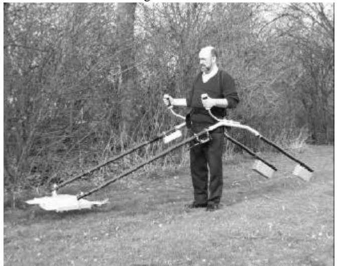
Fig. 2: Photograph of the DUNBLAD system. It is carried by the deminer using a comfortable harness. The audio signals from both detectors are clearly indistinguishable.
